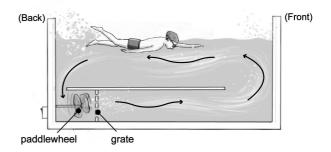
In the Mini-pool, no matter how hard one swims, the person goes 1 <u>nowhere</u>. The rear section of the aquatic exercise machine has a paddlewheel — 2 <u>separated</u> from the swimming area by a heavy grate — that propels water 3 <u>backward</u> in a channel under the bottom of the swim area. The constant current of water then resurfaces when it enters the 4 <u>front</u> of the swim area. And then it flows back 5 against the swimmer.
